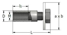
Fixing bolt anchor BBP consists of a threaded bush locked on a standard bolt and an anchor plate. The threaded bush is manufactured from steel S355JO, electrolytic galvanised (EV) or hot-dipped galvanised (TV); the bolt is made of steel 8.8 with no coating and the plate is manufactured from steel S235, also with no coating. The threaded bush can also be made of stainless-steel W 1.4571 –AISI 316Ti (SS4).
